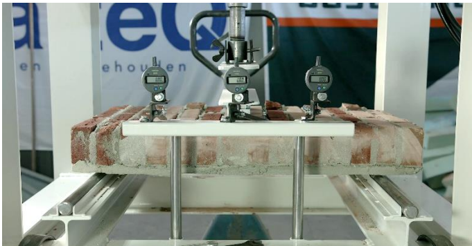
Figure 1. OOP test set-up
