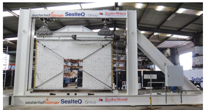
Figure 19. In plane test installation
